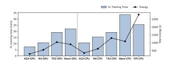
*Figure 5.* Flower enables quantifying the system performance of FL on mobile and embedded devices. Here we report the training times and energy consumption associated with running FL on CPUs and GPUs of various embedded devices.
