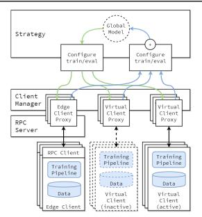
*Figure 2.* Flower core framework architecture with both Edge Client Engine and Virtual Client Engine. Edge clients live on real edge devices and communicate with the server over RPC. Virtual clients on the other hand consume close to zero resources when inactive and only load model and data into memory when the client is being selected for training or evaluation.
